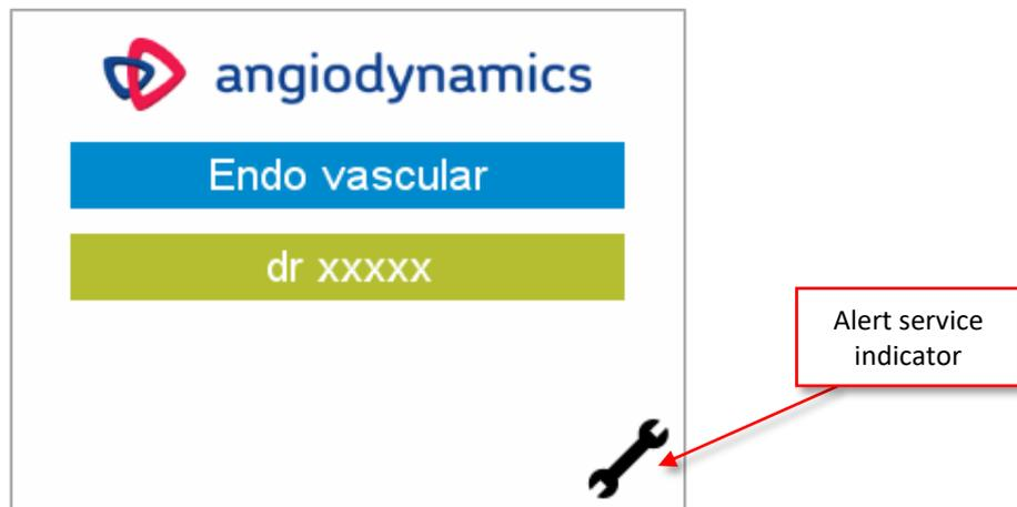
The *VenaCure 1470 Pro* laser should have an initial calibration check three years after the date of manufacture with subsequent annual calibration checks. If this check is due, a “wrench” symbol will be displayed on the program screen. This symbol will be removed after the calibration is completed.
