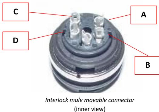
*The external door microswitch has to be connected to pins A and B. Contacts C and D close the signal lamp circuit (max current 1A, 24Vdc).*
