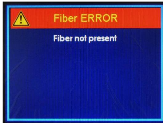
By entering in **Main menu** → **Diagnostics**, it is possible to see the error details. In the event of an Error, the Error message is displayed in red in the Diagnostics screen:
