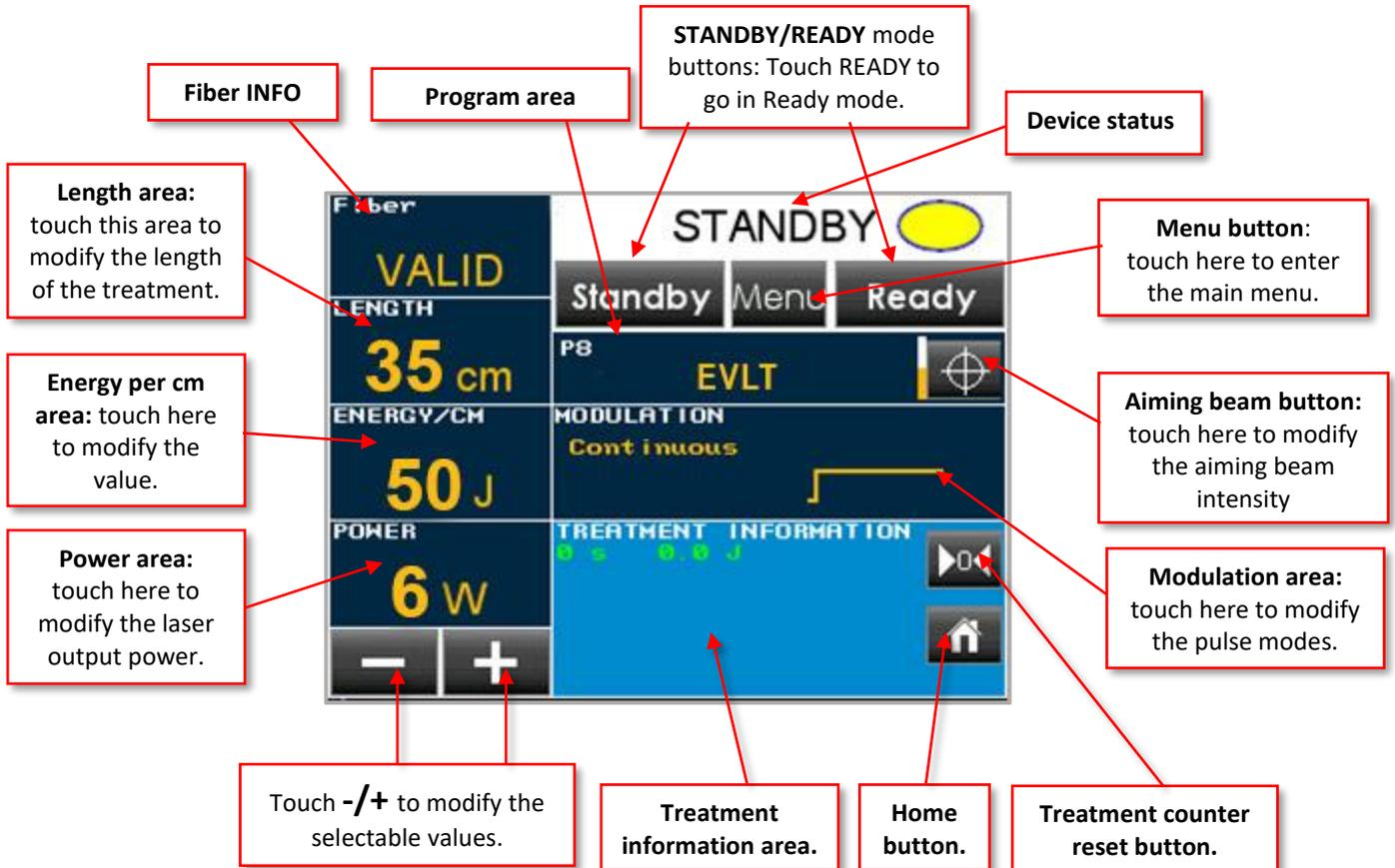
By selecting an area, its color turns yellow with blue values and allows to set the desired values with -/+ buttons.
