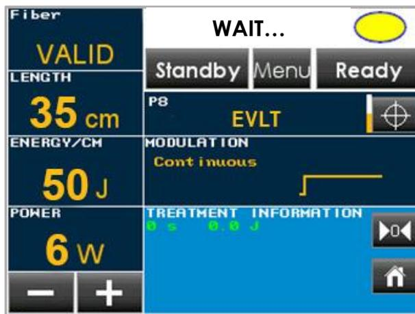
After a few seconds the system enter in READY status: in this status the user can enable laser emission by pressing the footswitch:
